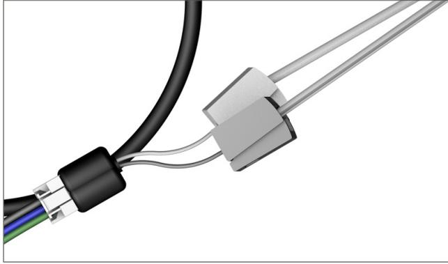
Connect the grey clip with the grey / white cable of the motor (-).
