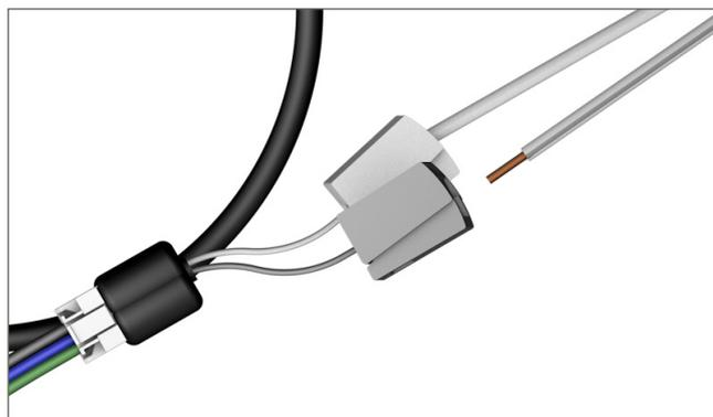
Regardless of the mounting position of the motor (left or right): Connect the white clip with the white wire of the motor (+).
