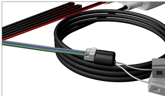
A. Put the programming plug of black cable and the motor connector together (grey / blue / green wire)
